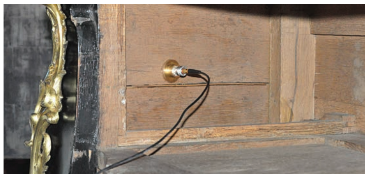
An eighteenth-century French commode displayed in the collection of the Victoria and Albert Museum. Photo: ©Victoria and Albert Museum, London. To monitor climate-induced fracturing of wood inside the commode, an acoustic emission sensor was mounted close to the tip of an existing crack. Photo: Marcin Strojceki, the Jerzy Haber Institute.
