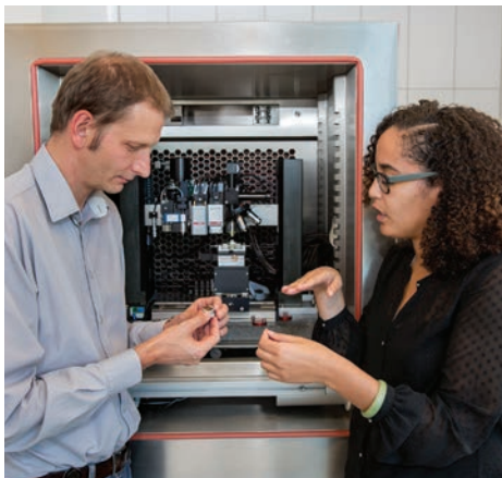
GCI Science staff Michal Lukomski and Ashley Freeman using the nano-indenter in a long-term study to better understand the response of hygroscopic materials to climatic fluctuations. Photo: Evan Guston, for the GCI.
